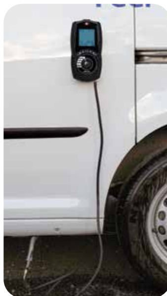
In cab heater CO 2 test with EP5 probe
