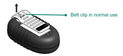
1. Lift belt clip at pivot end against the spring by a few millimeters then rotate 90 degree to clear battery compartment cover.
