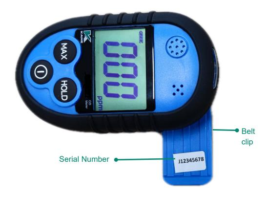
Enter KANE79 serial number in your analyser - once entered, readings are automatically sent whenever powered on & connected to your analyser
