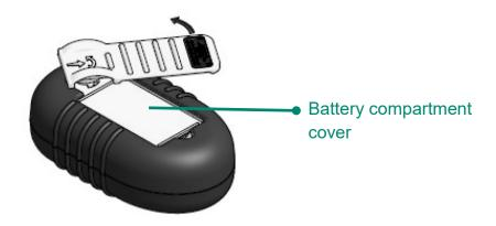
2. Remove cover and replace battery - We recommended alkaline batteries.
